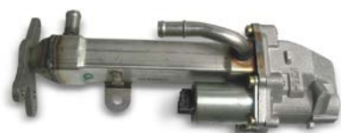
Fig. 1: EGR valve with EGR cooler
